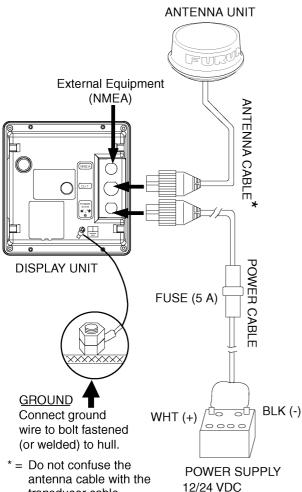
\* = Do not confuse the antenna cable with the transducer cable for the Echo Sounder LS-6100. The transducer cable is black; the antenna cable is white and "RADAR" is written on the cable.
